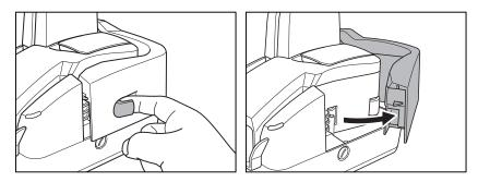
**2** While pushing down the open lever, open the reading unit.
